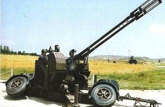
A photograph of an Oerlikon 35mm anti-aircraft gun. The gun is mounted on a four-wheeled carriage and has a long, angled barrel. It is positioned on a paved surface.                                                    |
